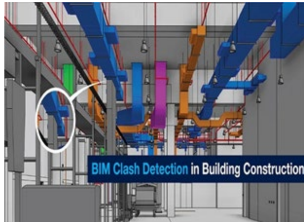
Figure 1: Illustrate examples of locations where clashes were identified through clash detection processes utilizing BIM
